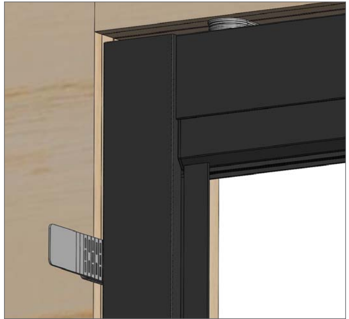
Shim Side Jamb against the Upper Channel & Top Track
