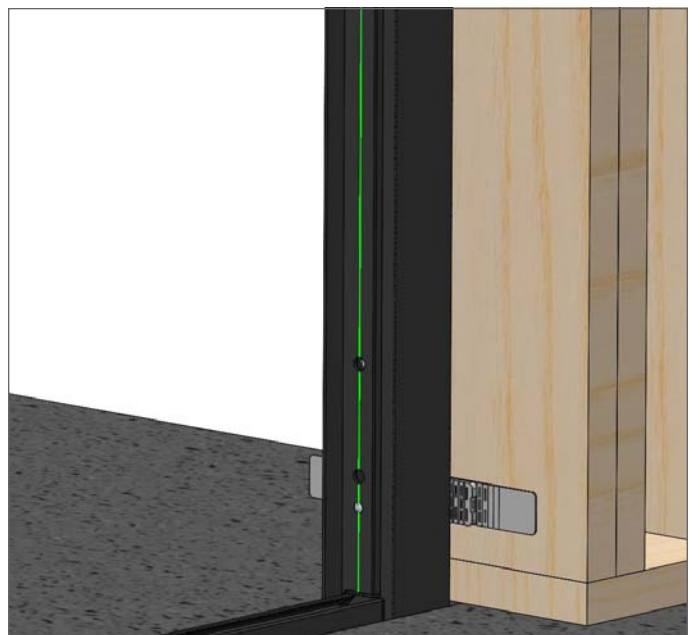
Check straightness with laser level and shim to adjust
