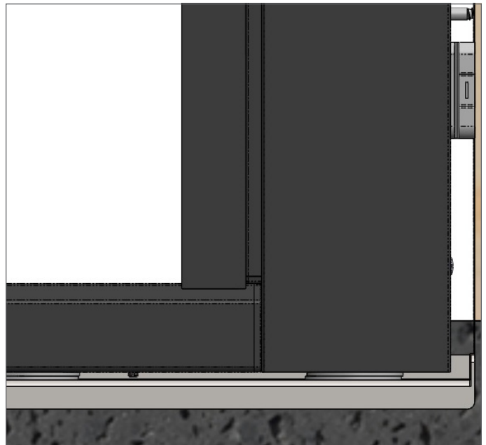
Lower Track End Cap is tight to Side Jamb
