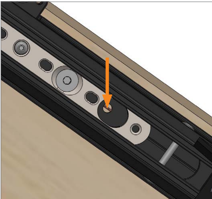
Upper Track fastener location, Daily Door side
