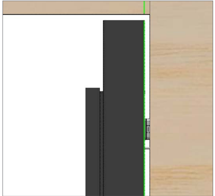
Shim top side of Side Jamb above the top fasteners
