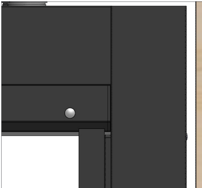
Upper Track End Cap and Channel are tight to Side Jamb
